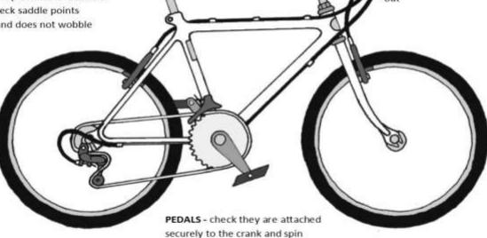
CHAIN & GEARS - check the chain is well oiled and not too tight/ loose. Check all the gears can be changed easily
